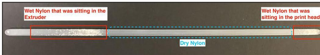
If your purge line appears to have more rough patches than described, consider running the utility again. Doing so will ensure that nearly all the filament in the second purge line will come from the drybox. If the second purge line also has a rough finish, then the filament in your drybox has likely been exposed to moisture.
