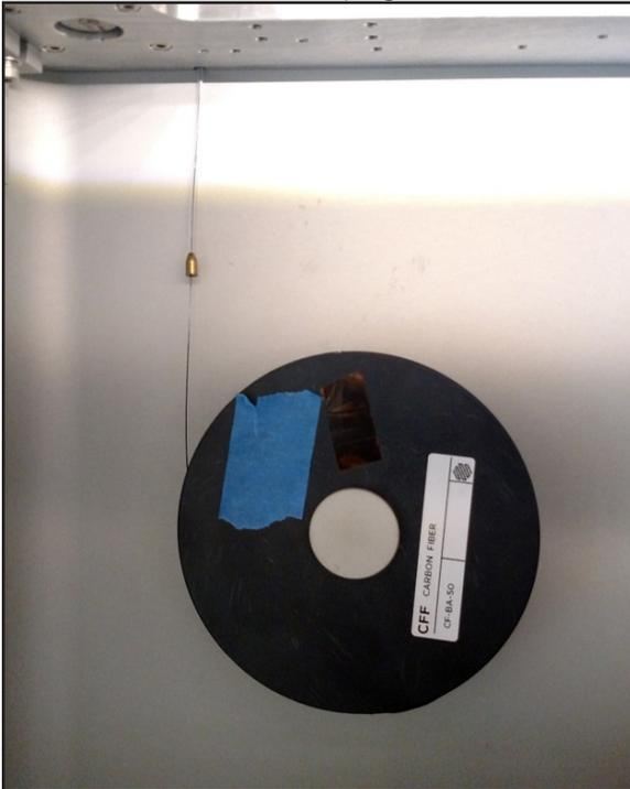
9. At the end of the Load Fiber routine, remove the cut piece of fiber from the print head.
