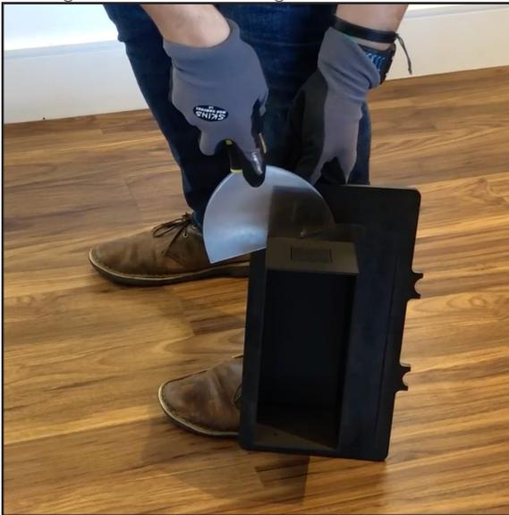
6. If the glue has dried, you can run warm water over it to rehydrate. Do not immerse the print bed or part in water.
