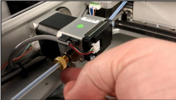
6. At the *print head end* of the Bowden tube, carefully insert the ferrule into the appropriate opening. Now screw the print head end tube retaining screw partway into the print head. Unscrew it, then finger-tighten the tube retaining screw into the print head.
