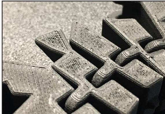
Typically, defects on vertical walls are *not* the result of underextrusion. If your printed parts have vertical wall defects and you are uncertain as to why, please contact Markforged Support.
