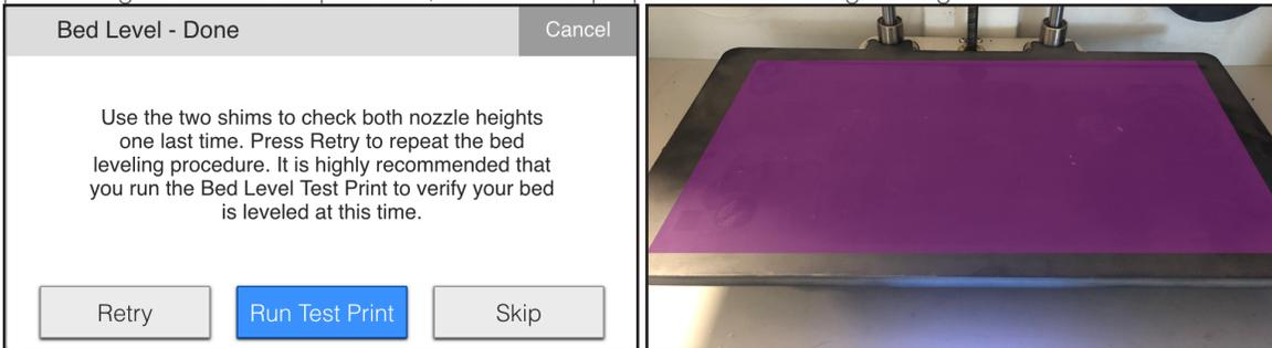
4. Run the Bed Level Test Print utility by pressing **Run Test Print** on the printer's touchscreen.
