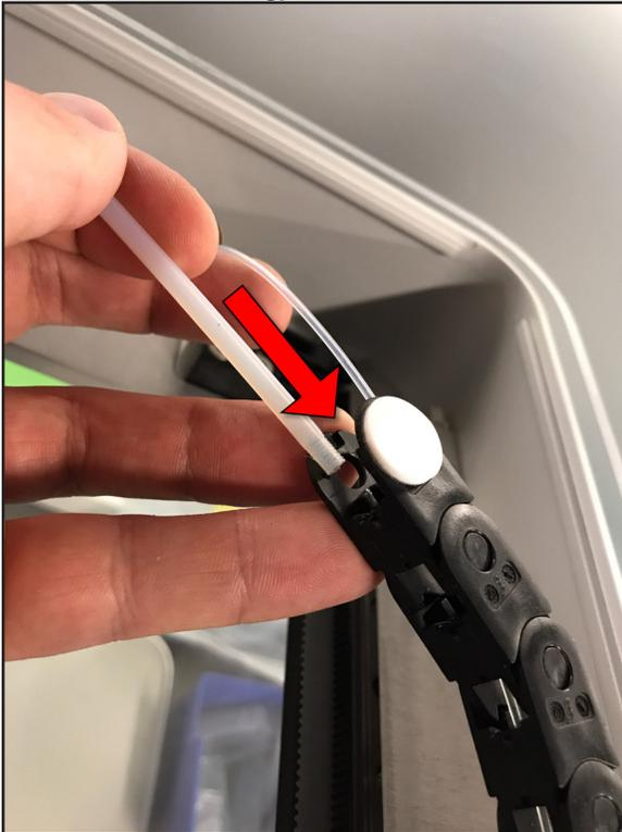
4. Once the Bowden tube passes all the way back through the energy chain, install the following hardware:
