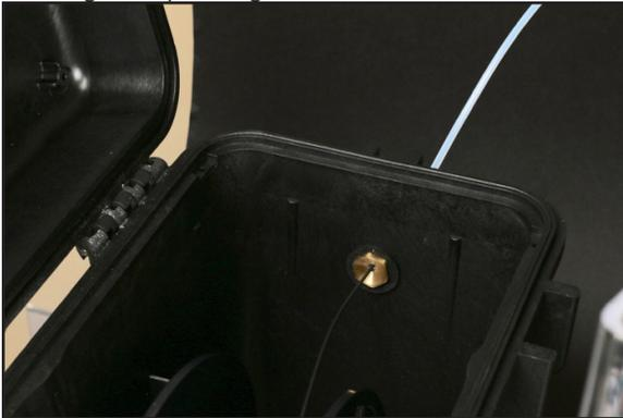
8. Feed the plastic feed tube through the opening in the back of your printer and let it hang freely.
