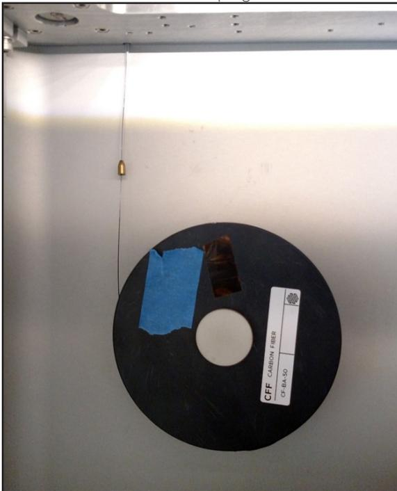
11. When the fiber begins to be extruded from the print head, press **Cut** on the printer's touchscreen.
