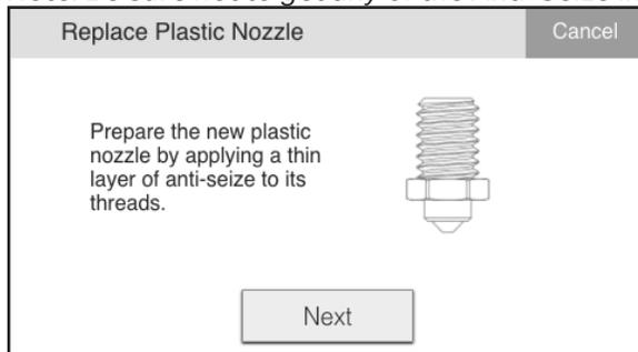
10. Using the torque wrench, screw the new nozzle partway into the print head, then unscrew it and screw it in again; this helps disperse the Anti-Seize over all of the threads.
